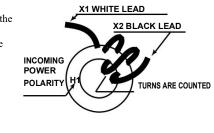
• To subtract secondary turns, the white lead should be wound through the CT from opposite the same side as the polarity mark.
